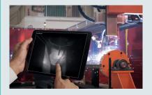
over shared networks. The addon to Xiris WeldStudio™ software allows many users to access the same live video stream using a tablet, smartphone, smart TV or PC with any compatible streaming software such as VLC media player for Windows, Linux, Apple or Android.
